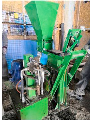
Fig. 2. Hydraulic static compaction device making earth-based brick like Ecorasillas.
