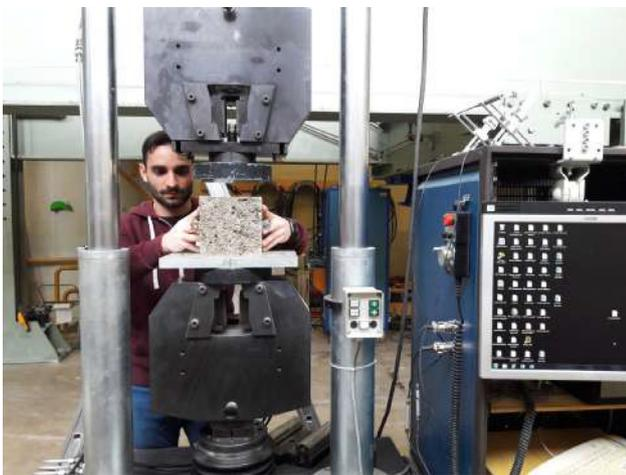
Fig. 10. Compression test setup.
