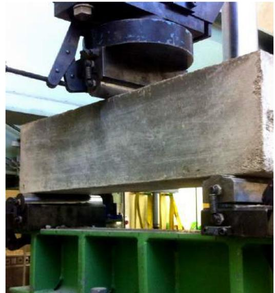
Fig. 16. Bending test setup.
