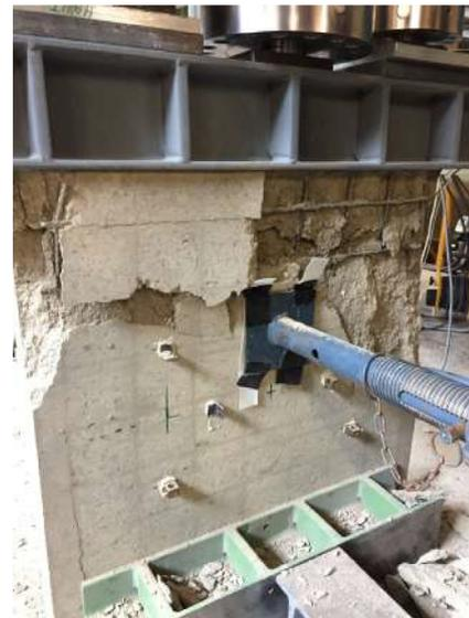
Fig. 20. Failure of the reinforced wall.
